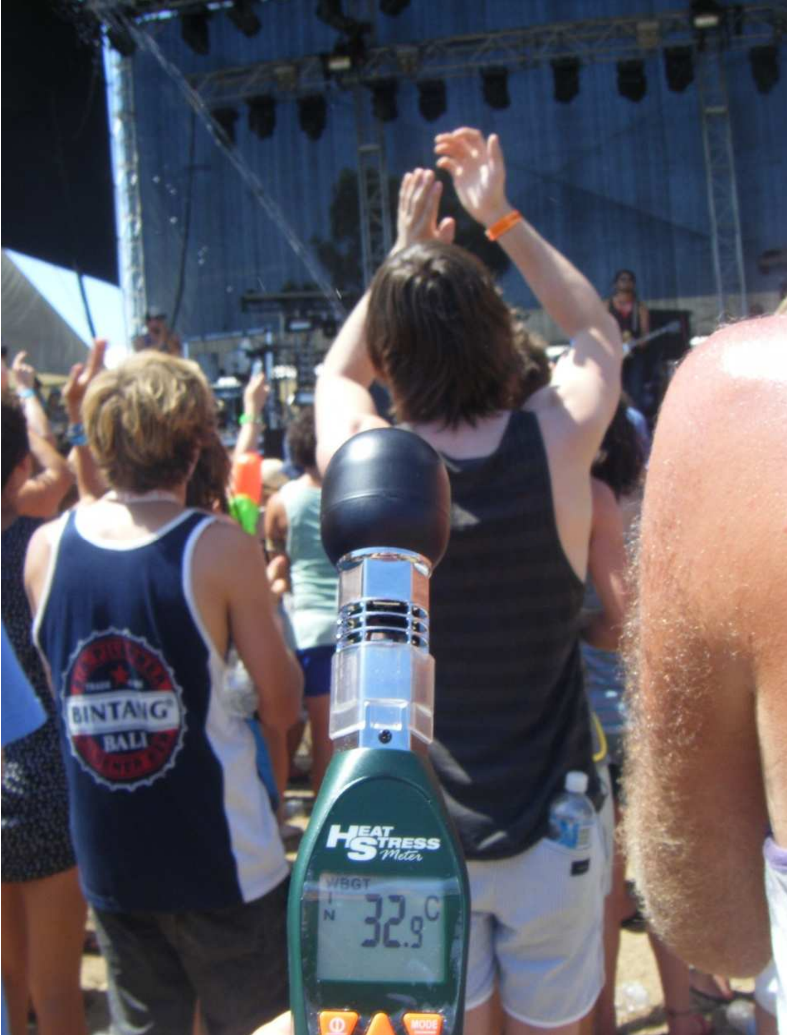
A heat stress metre used to monitor temperatures during visits to large outdoor music festivals and other mass gathering events
