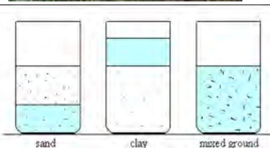
Figure 2 - Permeability of different types of soil components. In blue the distribution of water.
