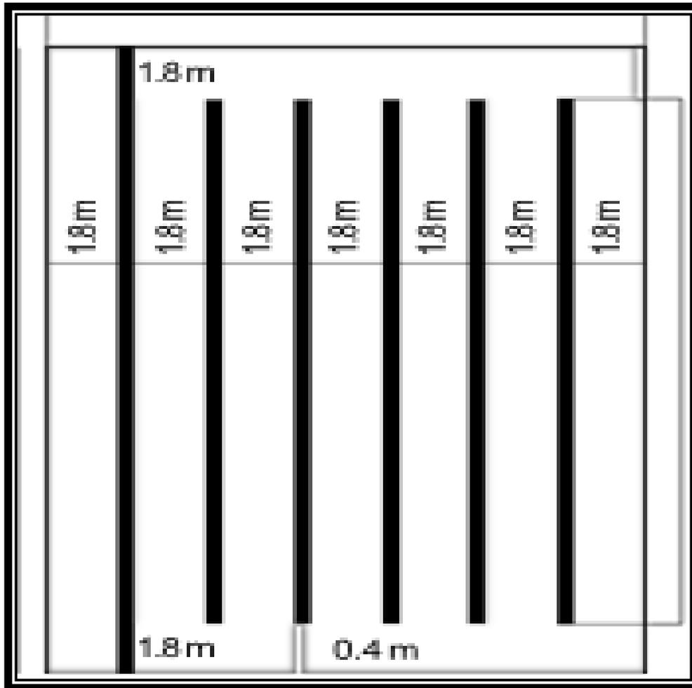
**Calculation:**  $900\text{L/d} / 20\text{mm/d} / 0.4\text{m}$  (width of the standard concrete leach drain 400mm) = 112.5 = 6 drains x 18.75m long
