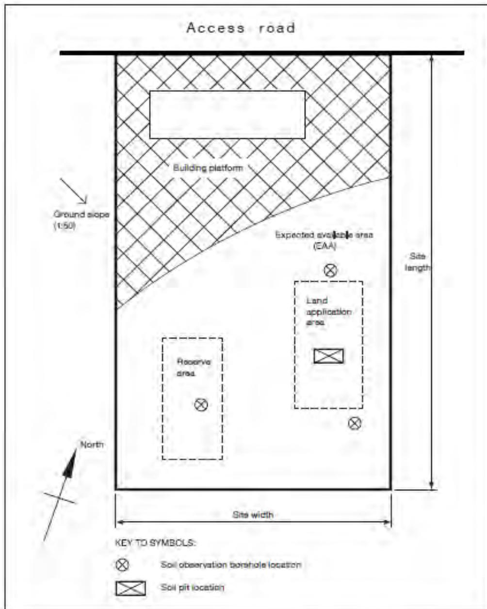
FIGURE D1 SITE PLAN - INDIVIDUAL LOT - EXAMPLE
