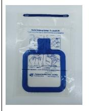
Used as a guide for 10 x 10cm sample area for **Aerobic Plate count and E.coli count** tests.
