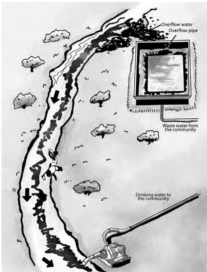
Fig. 2.41: This is how the overflow from sewage lagoon contaminates the community drinking water supply. This is the wrong way.
