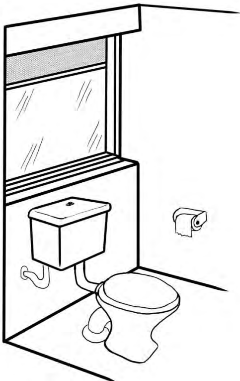
Fig. 3.6: A flush toilet with ventilation.
