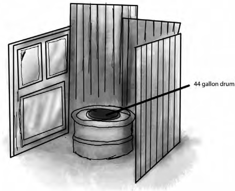
Fig. 2.2: Dry drop-hole toilet with roughly constructed seat and walls.
