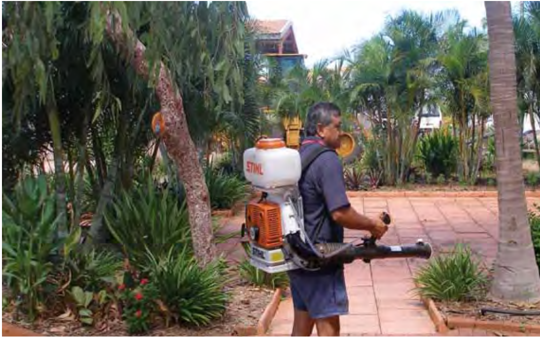
Fig 5.30: Motorised back pack sprayer
